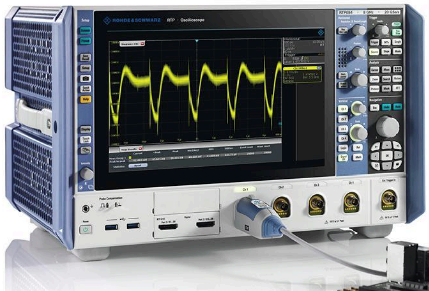
1. Low-noise, high-bandwidth scopes like the 8-GHz R&S RTP enable fast and accurate characterization of dc rails. Specialized probes designed specifically for power-rail measurements, such as the 4-GHz R&S RT-ZPR40 power-rail probe, have a number of attributes to produce high-accuracy measurements. (Source: Rohde & Schwarz)
